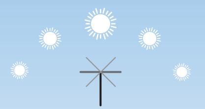
This technique starts working earlier than flat mounting solar panel and ends late in evening.
